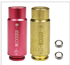
458 Socom boresight .length:38.3mm, bottom dia.13.7mm,top dia.12mm, color:brass/red
