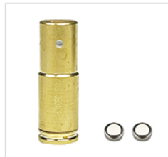
380ACP boresighter length:29.7mm, bottom dia. 9.5mm,top dia. 8.8mm
